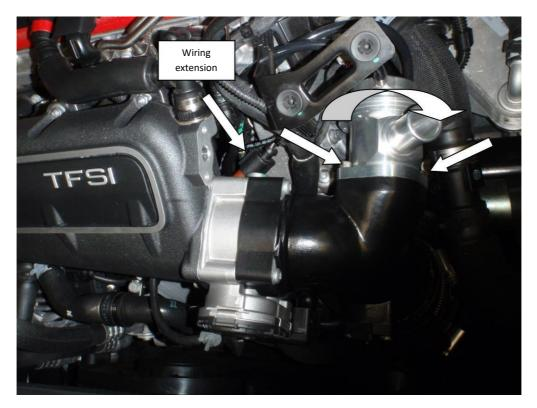
7. The Vacuum pump is located just above the gear box behind the gear box oil cooler. Cut through the small rubber pipe and install the T-piece supplied in the Kit.
