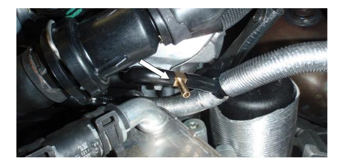
8. Forge highly recommend venting to atmosphere as this valve has a bigger bore for releasing the boost pressure. However, you can install this valve recirculating if you wish. Follow step one in reverse order and your installation is now complete.
