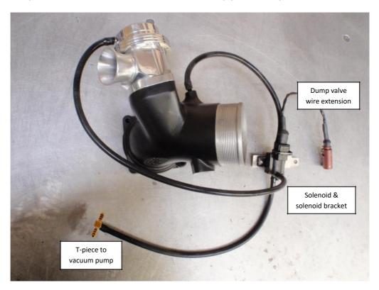
6. If there are any clearance issues when the high flow inlet and dump valve is fitted. Remove the dump valve with a 5mm Allen key, on the base of the flange you will see two small bolts undo with a 3mm Allen key. Rotate to the appropriate position and reattach dump valve.
